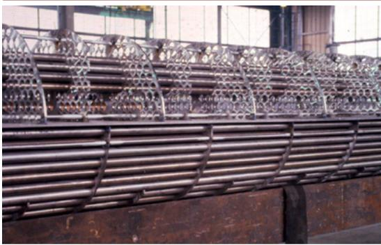
Segmental baffles used with two shellside passes.
