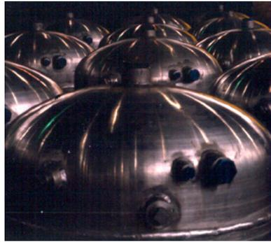
Aluminum hydraulic tanks used in hydrofoil boats.
