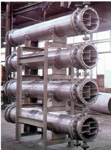
Nickel 200 8-pass, 4-shell heat exchanger.
