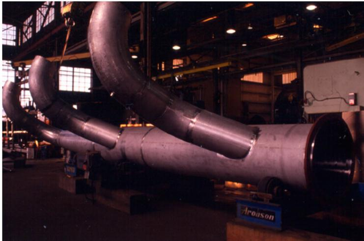
Piping header with polished internal surfaces.
