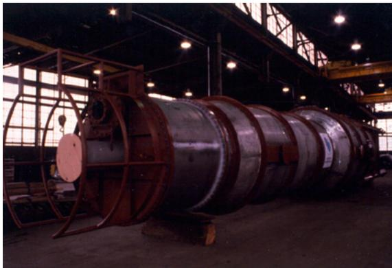
Stainless steel and titanium heat exchanger.
