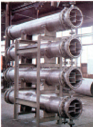
Nickel 200 8-pass, 4-shell heat exchanger.
