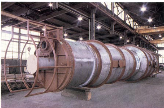
Stainless steel and titanium heat exchanger.
