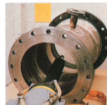
Radiographic inspection checks the integrity of welds.
